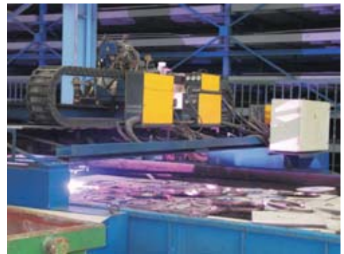
激光切割设备 Laser cutting equipment
