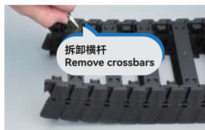
拆卸横杆 Remove crossbars 螺丝刀插入槽中利用杠杆运动撬开横杆 Insert screwdriver into the slot. Using a lever action, release the crossbars
