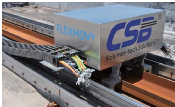
柔性电缆与拖链长行程户外滑行耐久测试 Long-travel outdoor sliding durability test for flexible cables and cable carriers
