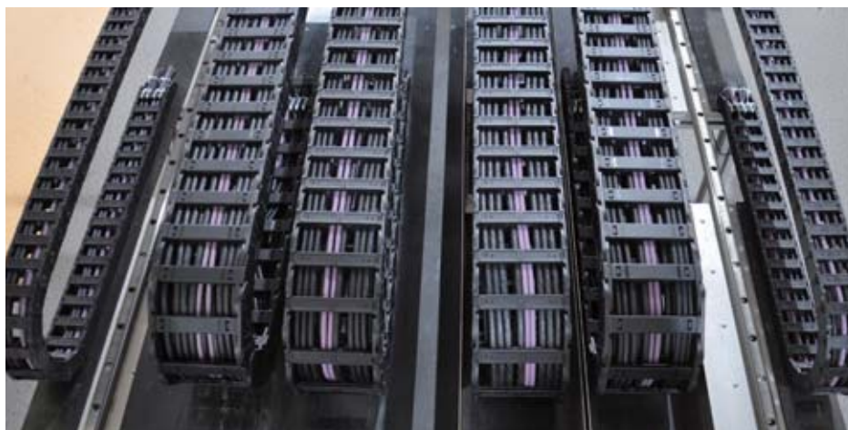
柔性电缆与拖链短行程架空耐久测试 Short-travel unsupported durability test for flexible cables and cable carriers
